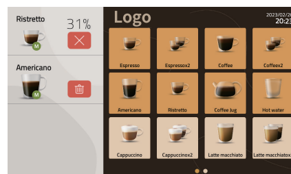
4. Queuing function can be used when beverage in preparation Touch Americano beverage icon when preparing Ristretto, Americano will be displayed in the queuing list as below.
