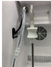
3. Connect milk hose (inlet) to mental milk hose
