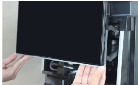
2. Lift the front operation panel
