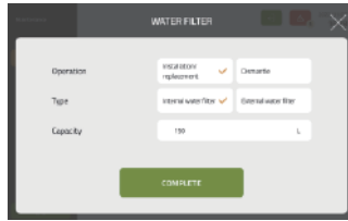
2. Select installation/replacement and internal water filter, input water capacity based on suitable level, then touch complete
