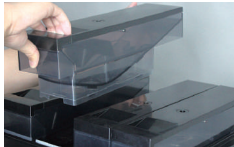
4. Remove bean hopper upwards
