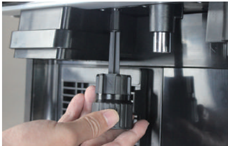
1. Use the key to unlock the operation panel (if need)
